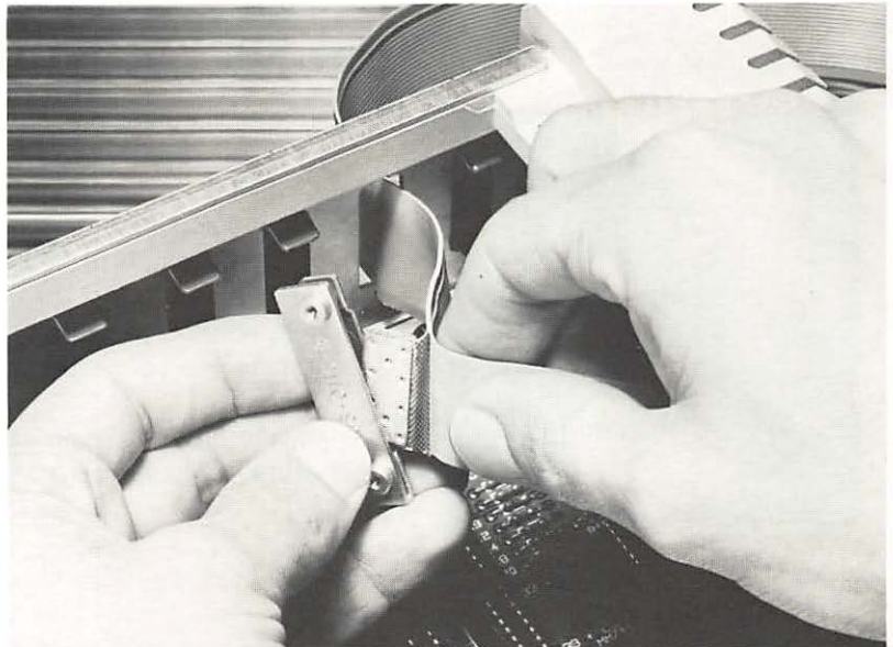
Figure 2-5. Place the Clamp Over the Metal Flap
