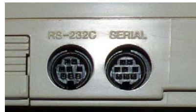
Figure 2: Left: Cable to connect the serial interface to a PC. Top: The Mini-DIN connector must have a small outer diameter to fit into the case.
